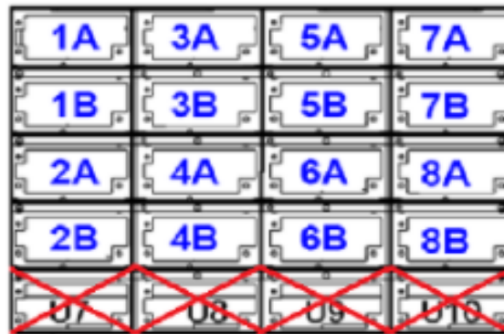
Figure A-1: Locations where the NAS70* cannot be installed
