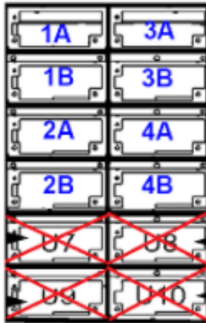
Figure A-1: Locations where the NAS70* cannot be installed
